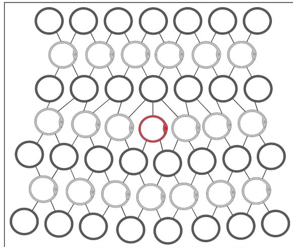
**Figure 16:** Representation of the use of an idle link to change the number of rings in a row. Drawing MA Wijnhoven.
