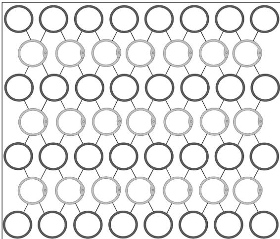
**Figure 4:** Representation of the 4-in-1 pattern with lines indicating which rings interconnect. The solid rings are shown in dark, and the riveted rings in light grey. Drawing MA Wijnhoven.
