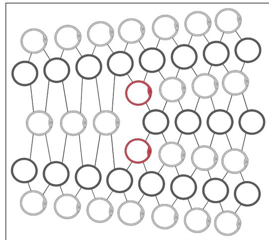
**Figure 17:** Representation of the use of idle links to change the number of rows. There are two manners in which idle links can be employed to this aim; one leaves a small hole, the other a knot. The former is illustrated here. Drawing MA Wijnhoven.
